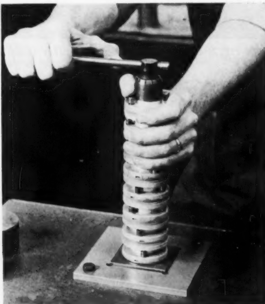
PRESSURE FIRMS BOND: Nut is tightened until bonding pressure is 35 psi. Oven curing is at 350°F.
